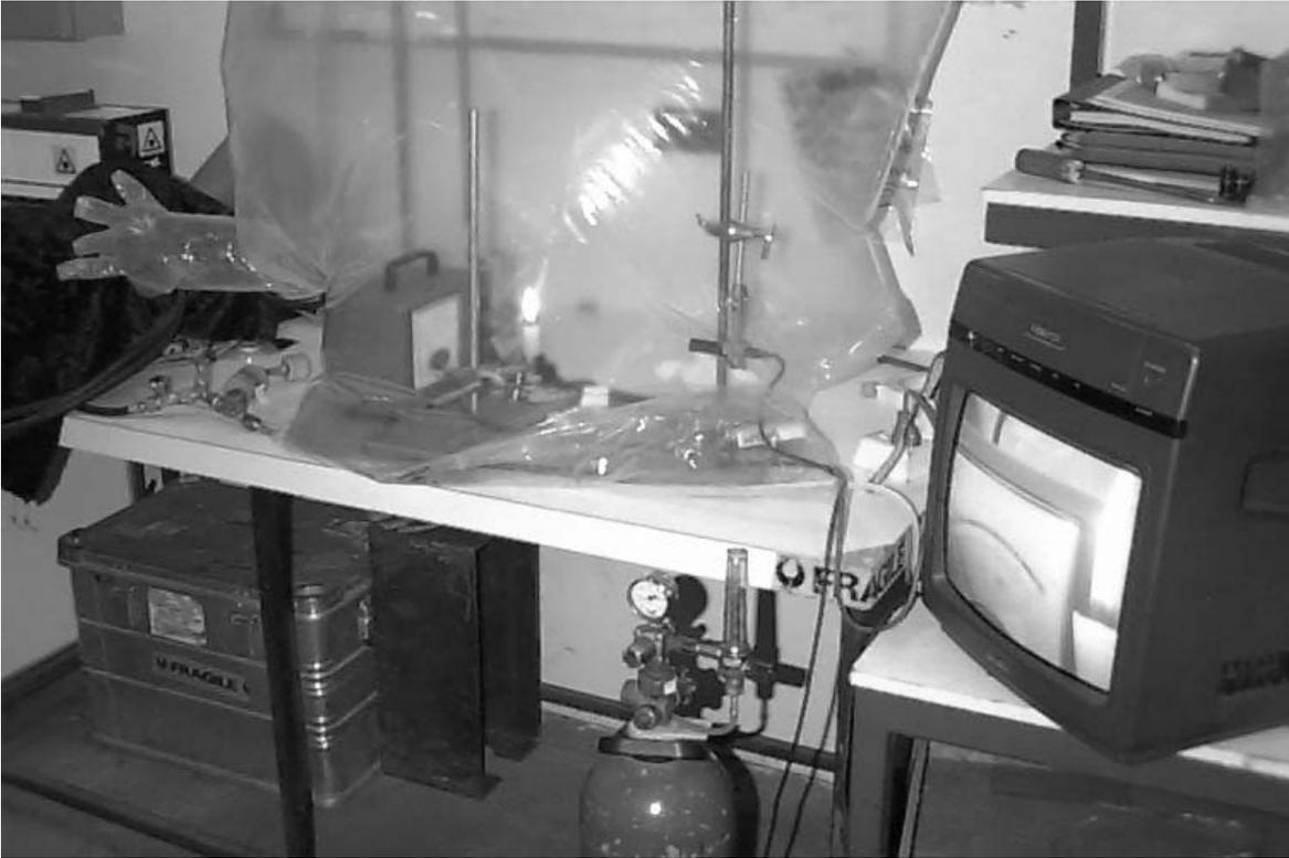
*Plate 1. Testing setup using a Teledyne Portable Oxygen Analyzer, and large inflatable glove chamber to measure oxygen concentrations which would extinguish various fuels. ie matches, candles and butane cigarette lighter.*
