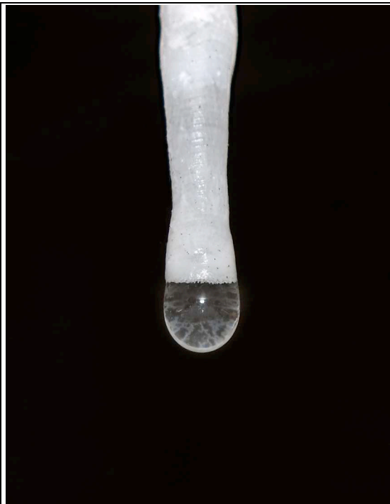
Figure 11: Slow drip rate increases calthemite straw diameter. Note the \text{CaCO}_3 rafts on the solution drop surface, which are a common feature at drip rates greater than approximately 12 minutes between drops.
