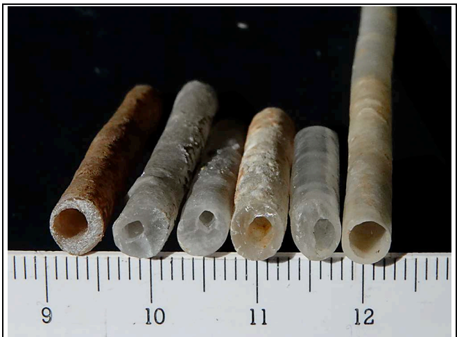
Figure 4: Typical cross sections of speleothem straws. Compare these with Figure 3. These straws have thicker walls and a denser crystal structure, making them less fragile than calthemite straws.
