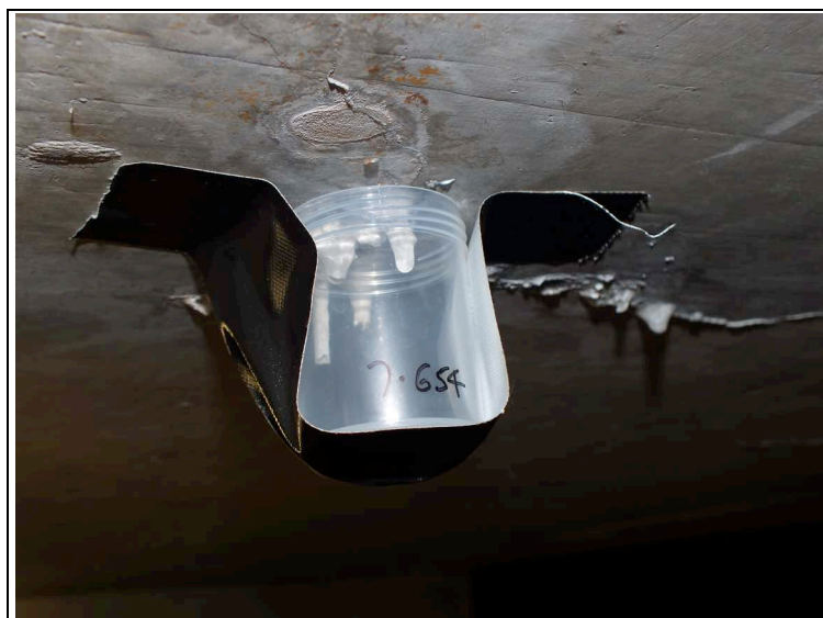
Figure 5: Gaffer tape holds the container against the underside of the concrete to collect the hyperalkaline solution dripping from a straw. The mass (in grams) of the clean container is written on its outside.
