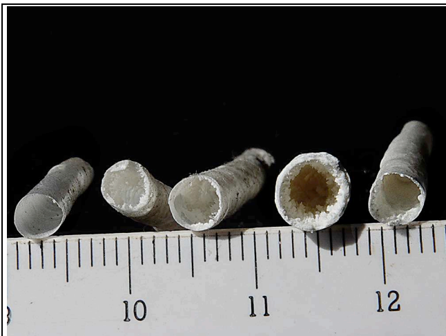
Figure 3: Typical cross-sections of calthemite straws. These have a thinner wall, are more fragile and have a less dense crystal structure than do speleothem straws. The image scale divisions are in mm.
