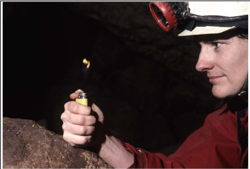
Jenny Whitby demonstrates how a naked flame from a butane cigarette lighter, burns remotely from the lighter jet when the oxygen content of the cave atmosphere is just sufficient to support combustion. Note in good air the flame extends right down to the lighter jet. There is no flame adjustment on this lighter. Photo Garry K. Smith
