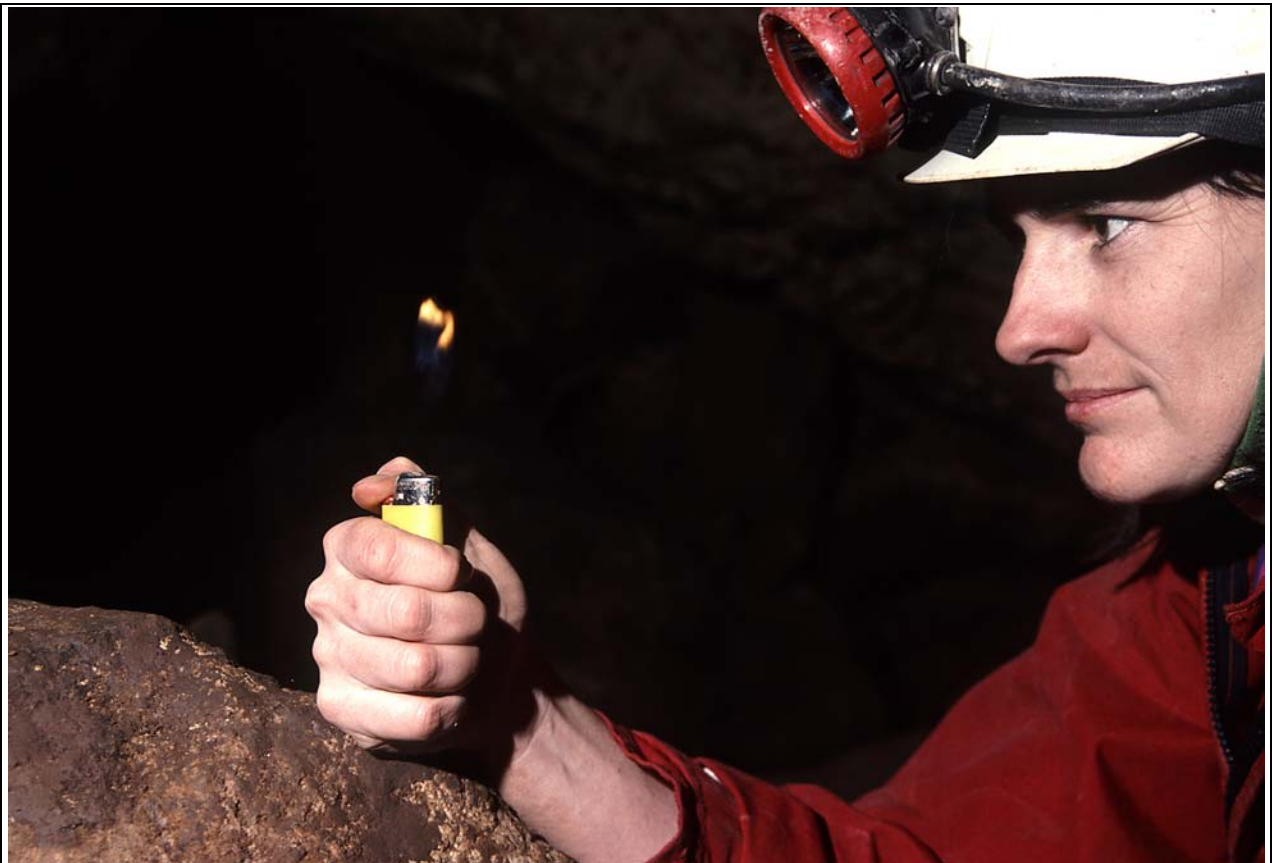
Jenny Whitby in Grill Cave, Bungonia NSW. Australia performs the flame test for foul air. The CO 2 on this occasion was measured at 5% with a Drager Meter. Photo by Garry K. Smith ©.
